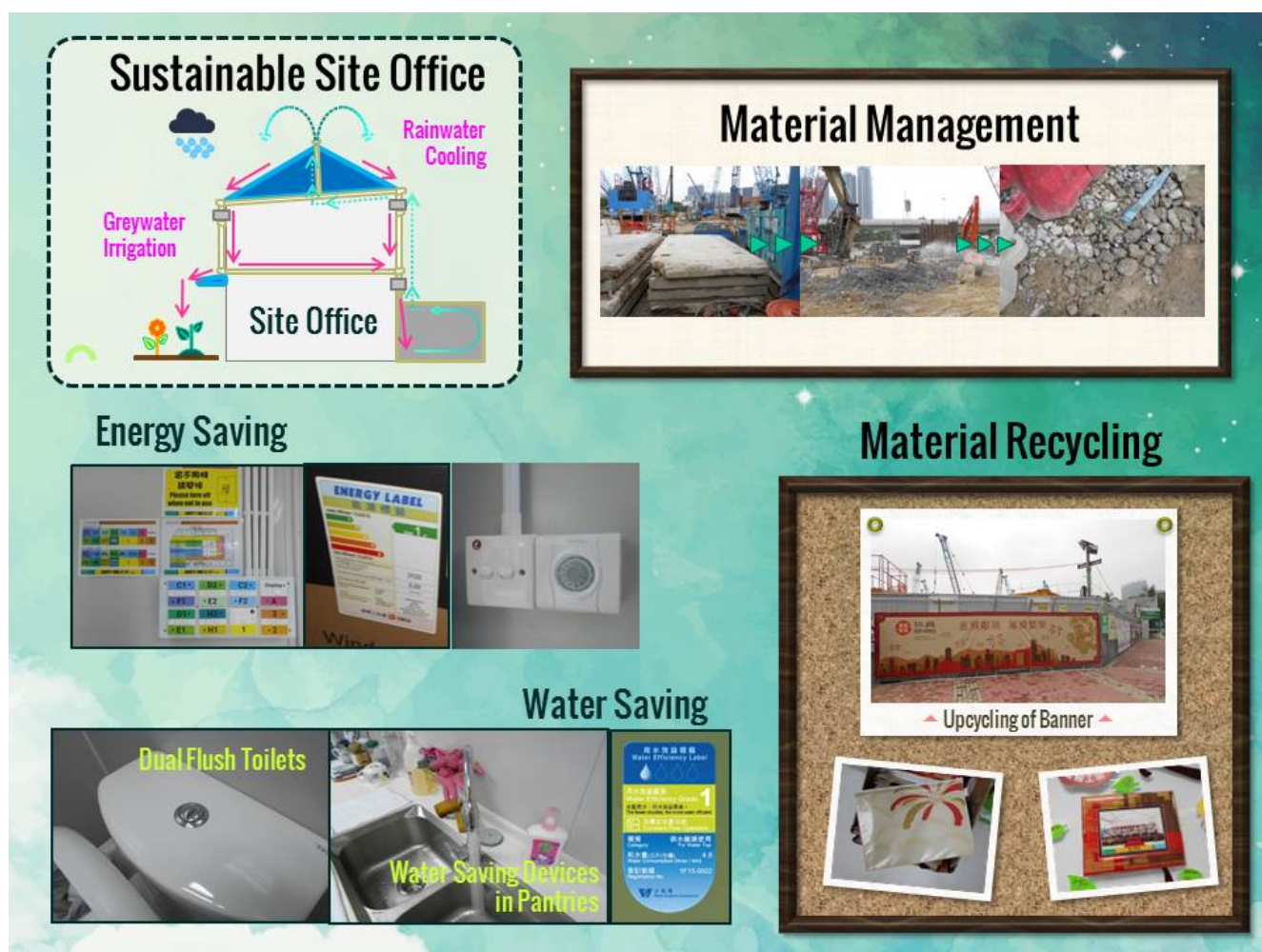
Green/ Environmental Measures carried out during the construction of WKGO
