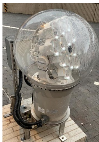
Sunlight collector at WKGO
